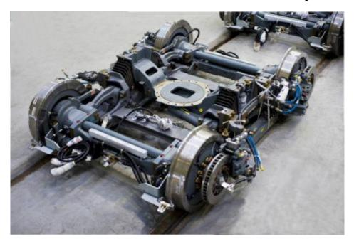
Our global solution is composed of primary suspensions, secondary suspensions, laminated bushes, stops, and coupling. It stabilizes the rain on the tracks and provide vibrations insulation to optimize the comfort of passengers.
