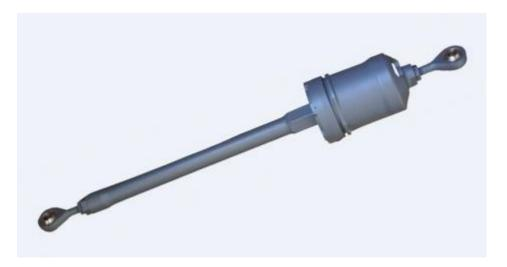
Our Lead-Lag Dampers are installed on helicopter rotor heads either between the hub and the blade or between two consecutives blades. They're essential rotor components that ensure dynamic stability of the aircraft under all operating conditions. These solutions are especially critical for preventing ground and air resonance.
